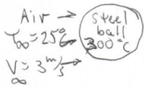
Then blow air at 1 atm &  $25^{\circ}\text{C}$  over it at  $3 \frac{\text{m}}{\text{s}}$ .Eventually  $T_{\text{surf}} = 200^{\circ}\text{C}$ ,
