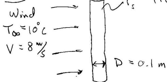
Calculate rate of heat loss per unit length.
